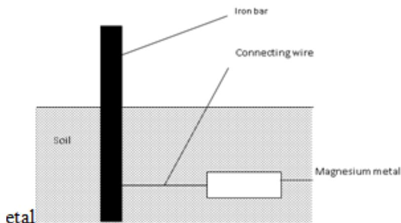
Explain why it is necessary to connect the piece of magnesium metal to the iron bar. (2mks)
